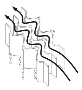
98 Effective at Removing salt splay and Water from Engineroom Intake Aiv
